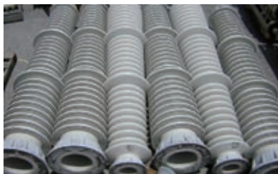
Damaged ceramic insulators are recycled into material for tiles.
