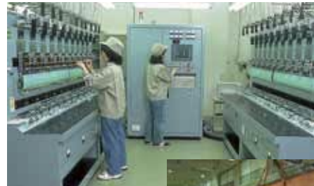
Employees of Okinawa Denki Kogyo Company, Incorporated check power meters.
